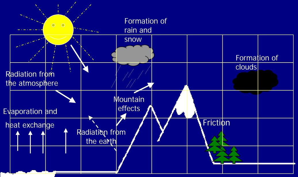
The atmosphere is split up into a 3-D grid. Each land based grid is about 60km.
