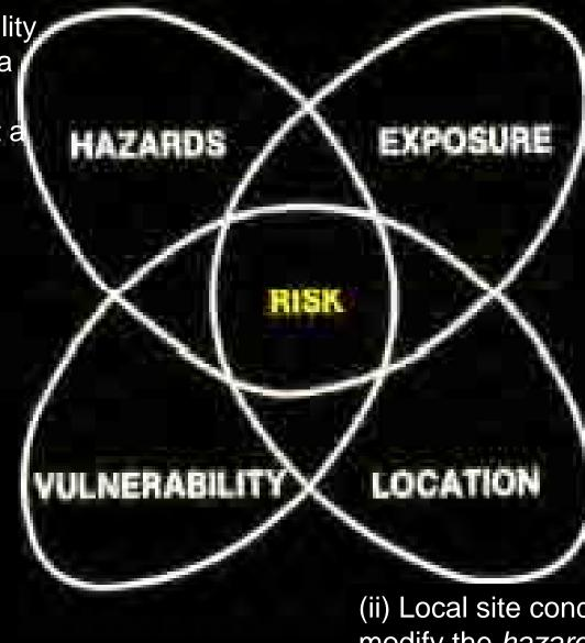
**EXPOSURE**- Objects and structures built by man which are exposed to the effects of the `*hazard*': buildings, bridges, dams, power plant, life-line structure, etc.
